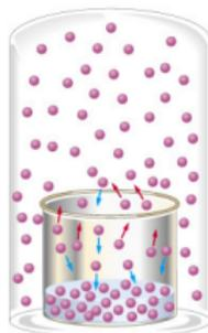
(c) Vaporization rate = condensation rate
